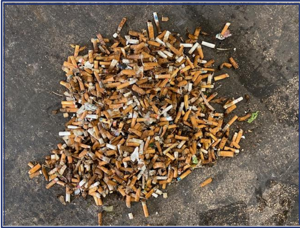
Figure 26. Cigarette butts found in a sample after further analysis of the undersize fraction
